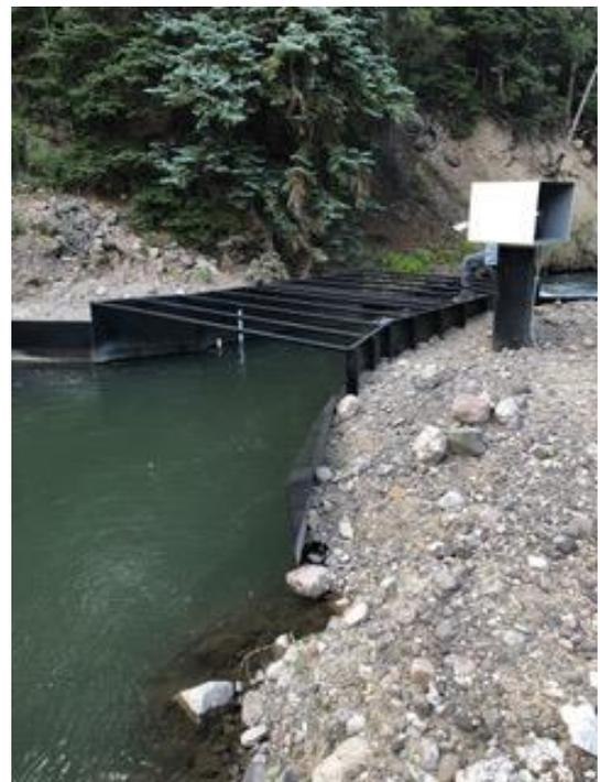
Flume with automated level sensor.
